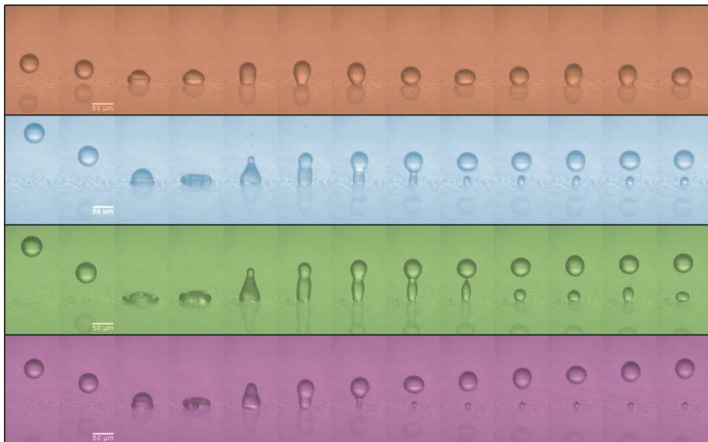
Droplets impacting a nanoparticle coated glass surface, increasing in speed from top row to bottom. From 2m/s to 7m/s, each image taken 0.01ms apart.
