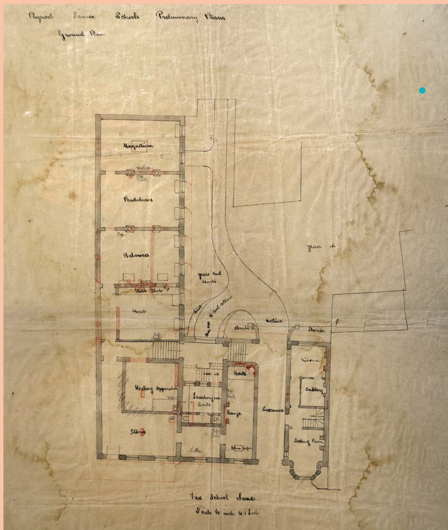
Fawcett's plan for the ground floor of Cavendish Laboratory with Maxwell's changes indicated in his own hand in red pencil.
