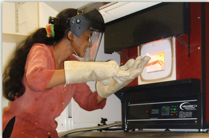
Fig. 5: High temperature furnace used in the laboratory for the preparation of single crystals by the flux growth technique.
