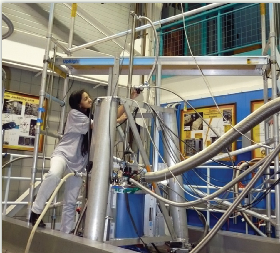
Fig. 2: World's highest field hybrid magnet combining resistive and superconducting technologies to reach continuous magnetic fields of 45 T in the National High Magnetic Field Laboratory, Tallahassee, Florida.
