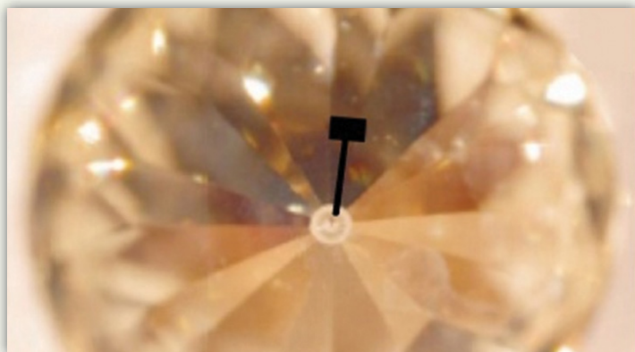
Fig. 6: A diamond anvil for high pressure research with inset microcoil of size \approx 0.3\text{mm} .
