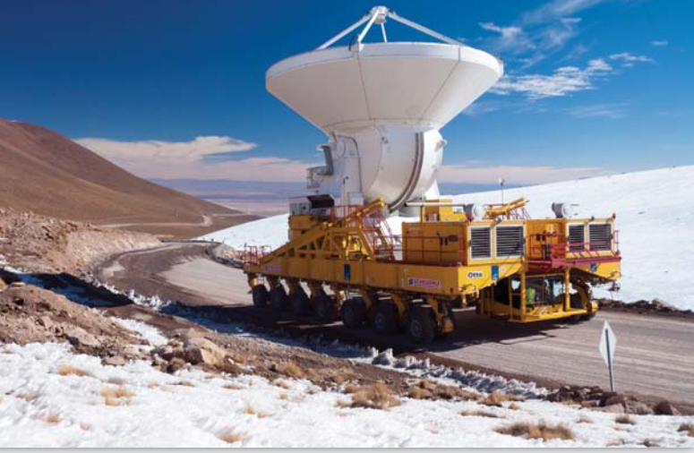
Fig. 2: Antenna 16, the first European 12-metre antenna, on the transporter from the ALMA Operations Support Facility at 2900 metres to the summit plateau at 5000 metres.
