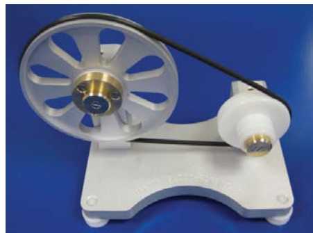
Martin Blood-Forsyth with the product of the workshop training project. Each student built their own version of this drive mechanism.
