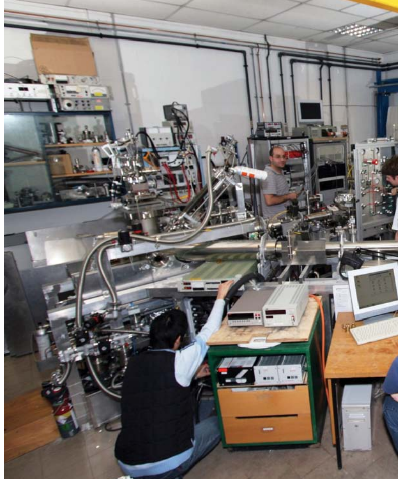
Fig. 1: The HeSE apparatus consists of a long V-shaped vacuum system. The high intensity source is on the left and the detector on the right. Development of the HeSE technique was a major project in the Cavendish workshop facilities. The instrument is fully automated and typically runs 24 hours a day.
