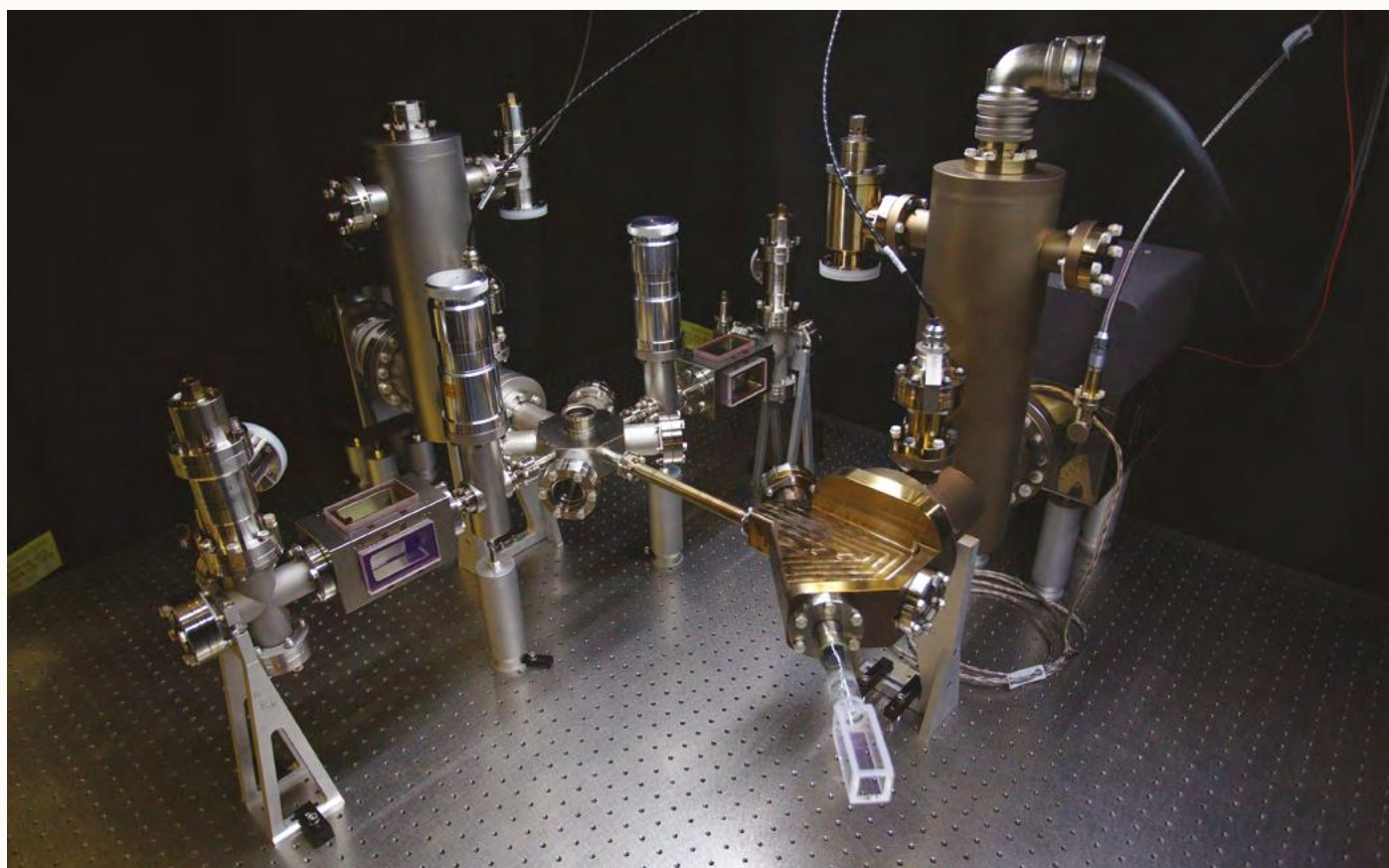
FIG 3. The vacuum system for ultracold quantum gases used in the experiment.
