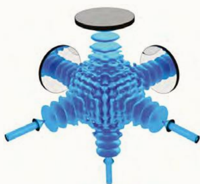
FIG 2. Illustration of the equipotential surface of a 3D optical lattice formed by reflected standing wave laser beams.
