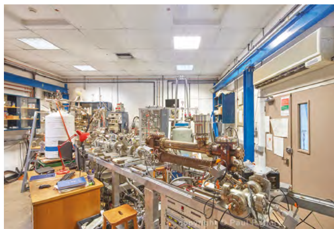
FIG. 1. The Helium Spin-echo (HeSE) Microscope of the Cambridge Atom Scattering Centre. Photograph © Paul Raftery courtesy of Bougyues UK
