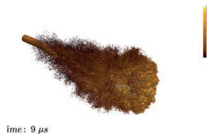
Figure 1. Jet breakup and preferential evaporation of a multi-component fuel.
