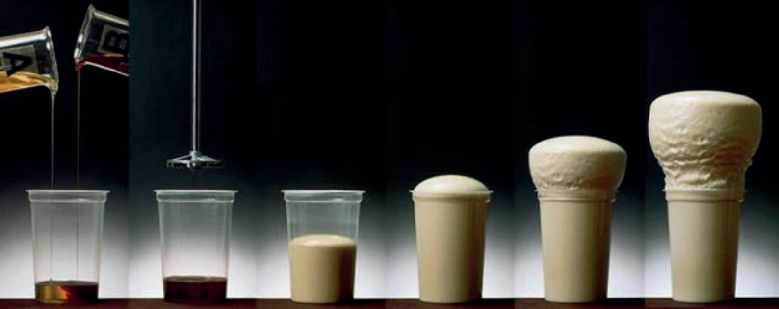
Figure 3. Production of polyurethane foam involves multiple scales: chemical kinetics models, bubble growth and pseudo-fluid model at the scale of the final product.
