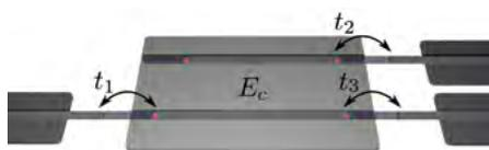
**ABOVE:** The minimal setup to detect the topological Kondo effect. Majorana fermions (red dots) are envisioned here as emerging in spin-orbit nanowires (horizontal bars) coupled to a superconductor (central rectangle). The outermost wire segments form leads of conduction electrons, tunnel coupled to three of the four Majorana fermions.
